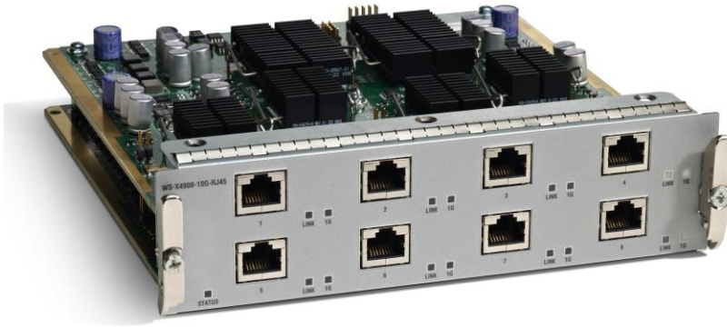
Figure 5. 8-Port (2:1) 10GBASE-T RJ-45 Half Card 1 (Capable of Operating at 1G/10G for Up to 100m on Cat6a/Cat7 Cable)
